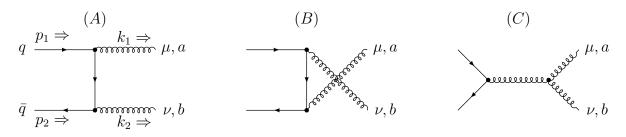
Here  $p_1, p_2$  are the momenta of the incoming quark, anti-quark with  $p_i^2 = m^2$  and a, b = 1, ..., 8 are the color indices of the outgoing gluons with momenta  $k_1, k_2$  and  $k_i^2 = 0$ .
